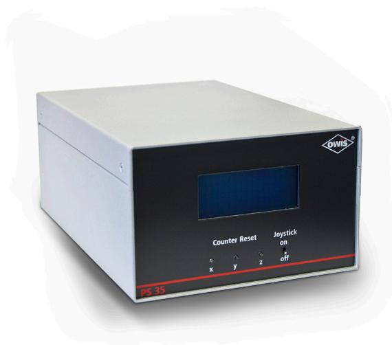
The PS 35 as an universal position control unit in a table top with LCD controls up to three axes of 2 phase step motors or DC servo motors (brush). Different combinations of both motor types are possible. The display shows the status of each axis and its position with measuring unit. Further, for each axis a reset button is provided.
