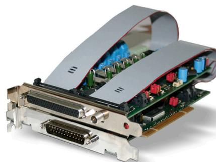
The OWIS PS30 is an universal position control unit for installation in a PC. It consists of a plug-in card and an output stage module without PCI connector, mounted on a second slot panel (short PCI format 106 x 168 mm). Both cards are flexibly connected by a flat ribbon cable.
